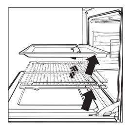
When pushing the tray, pan and rack back in, always ensure that the safety notches are at the rear of the oven. (See illustration)
